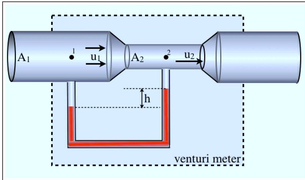
Figure 1: Illustration of a venturi meter.
