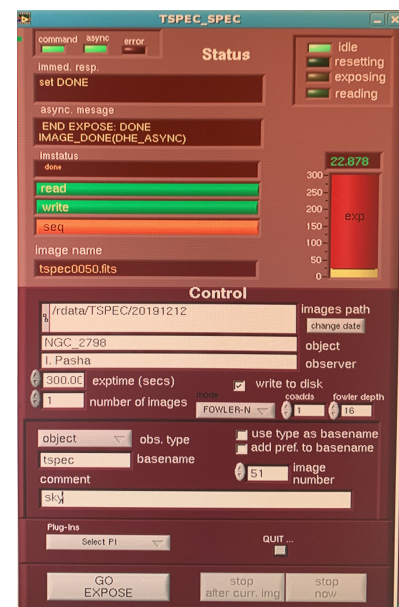
Figure 4: The TSPEC_SPEC window. 3 When you are ready for cals, confirm the dome is dark with the Telescope Operator (TO) and then, after taking darks, ask them to turn the high lamps on for flats.
